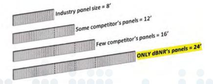
In order to realize exceptional savings on field installation time and labor, reduce the number of structural steel supports, and to further refine architectural appearance and quality, dBNR Nois-eNvelope™ systems have optimized the maximum panel length to 24 ft. (7.32 m.) span, which is 2-3 times the length of most competitors' panels.
